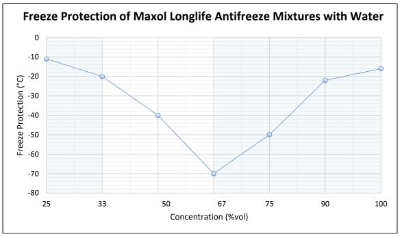
Freezing Protection = Average of Freezing Point (ASTM D1177) and Pour Point (ASTM D97)
