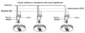
NOTE: Use standard British Standard household cable PVC/PVC 6242Y / 6243Y or equivalent in accordance with local regulations.
